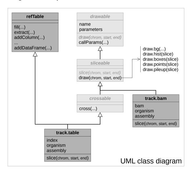
Rgb heavily relies on class inheritance to avoid code duplication. As can be seen on the UML diagram above, objects from the track.table class (most of the objects manipulated in Rgb) are a convergence between the refTable class (that stores tabular data in an efficient way) and drawable-inheriting classes (managing all the drawing process, independently from the data type).
